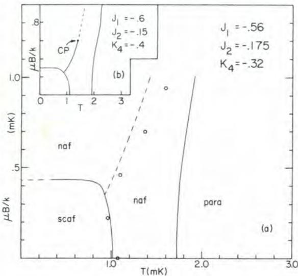
FIG. 1. (a) Phase diagram of  $^3\text{He}$  below 3 mK as determined by experiment of Ref. 7 (open circles) and according to mean-field theory based on coefficients shown. (b) Inset shows how first-order transition with critical point (CP) can be obtained with slight adjustment of parameters.
